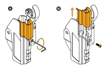
To prevent dust from entering, insert the SH14 Plug and secure it by tightening the screw clockwise.
